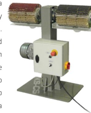
of sanding applications. Additionally, the speed and rotation sanding heads can be controlled by the variable frequency drive. Two 100mm (4") dust ports keep the dust contained for a clean working environment.
