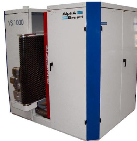
hang-lines allowing you to process parts without taking them off the hang-line. The Alpha-Brush vertical machine uses a variety of rotating and oscillating discs and is adjustable for disc height, rotation speed, oscillation speed and conveyor feed speed. Let Alpha-Brush work with you to design and implement the best vertical brush solution for your needs.
