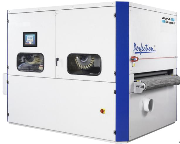
The Alpha-Brush *Perfection* line of brush sanders are top of the line! These patented brush sanding machines can be ordered in a wide variety of sizes and configurations. Due to the variety of specific designs the brush machines integrate perfectly into a wide variety of applications in the wood market, metal processing, plastics, composites and more. These heavy-duty machines are designed and built to be run 24/7 in the most demanding conditions. The
