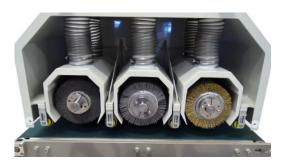
The KS-WBM is equipped with three top sanding heads with a conveyor designed to process one side in a single pass. The machine can handle parts up to 400mm width (16"), but is open in one side to allow wider parts to go through. Six 100mm (4") dust ports keep the dust contained for a clean working environment.
